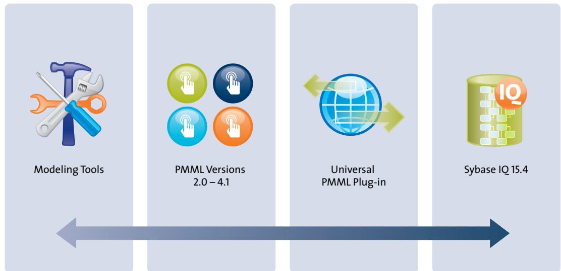
Figure 2. Developers can use their tools of choice and export their models into a PMML standard file, then use the Sybase Universal PMML Plug-In to run the model in Sybase IQ.
